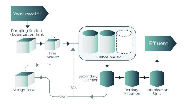
Aeration processes used to degrade organic matter represents anywhere from 25 to 60 percent of a traditional wastewater treatment plant's energy expenditure. Using passive aeration, MABRs demonstrate a dramatic 87 percent reduction in aeration energy consumption compared to conventional activated sludge (CAS) processes that employ diffusers and high-powered blowers (see table below).
