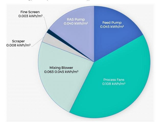
**Energy Consumption Breakdown of a Typical MABR Treatment Process**
