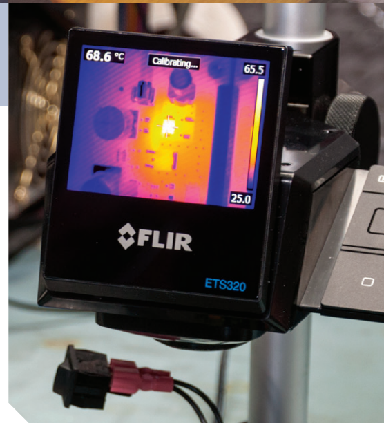
With 76,800 points of non-contact measurement and thermal sensitivity of <math><0.06^{\circ}\text{C}</math>, the FLIR ETS320 helps engineers quickly identify design flaws.
