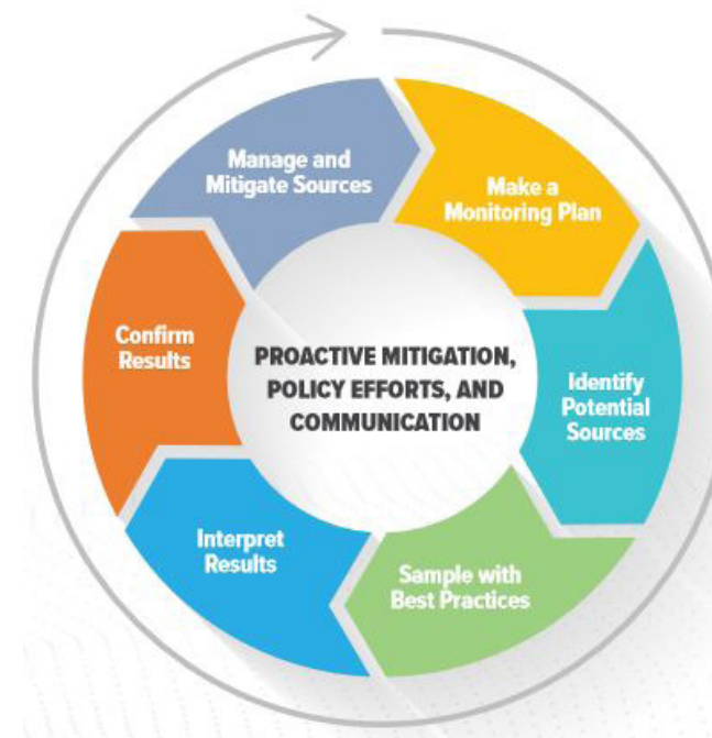
Figure 2 - Step-by-step guidance for source tracking of PFAS.
