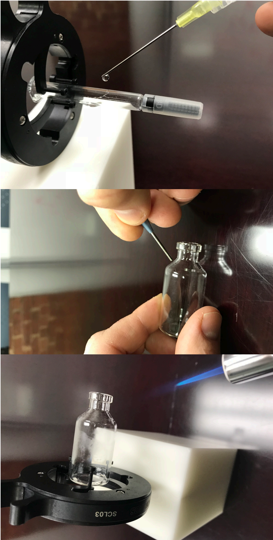
Figure 2 Scratching Process to Test Glass
