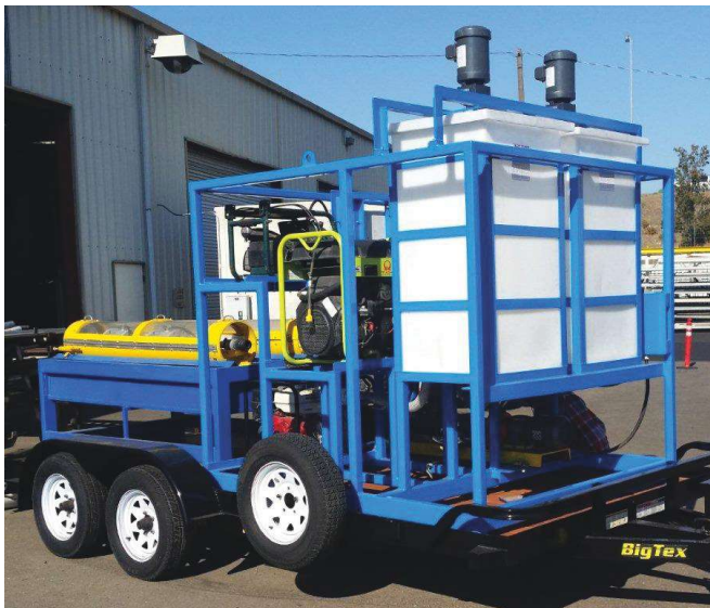
Forward progress: Tangential flow separators can be small and transportable, as shown, or scaled up for large flows.
