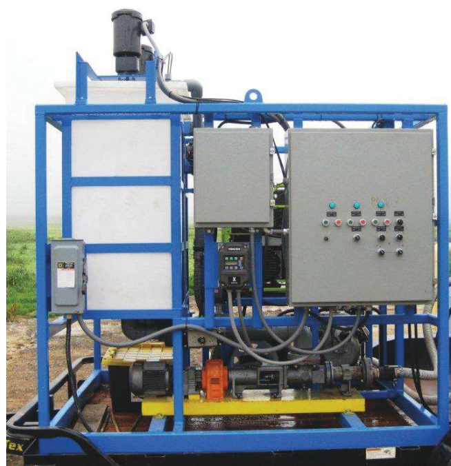
Advanced controls optimize the performance of the tangential flow separator’s physical processes.
