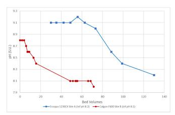
Figure 2. pH vs. bed volumes (data from single-pass rinsing [not recirculated]) (Source: Jacobs)
