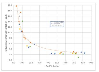
Figure 3. Arsenic concentration vs. bed volume from bituminous GAC startups (Source: Jacobs)
