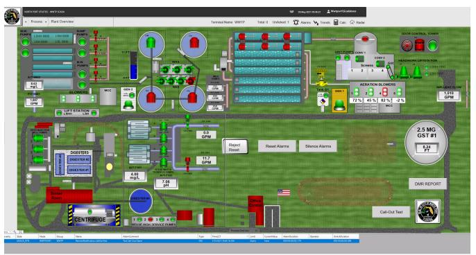
Overview of the city's wastewater equipment connected to remote alarm notification software. When an alarm occurs on specific equipment, the City of North Port can visualize the alarms through its SCADA system
