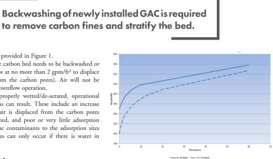
Figure 1. Example wetting curves for 8x30 and 12x40 mesh bituminous GAC Source: Calgon Carbon Corporation)
