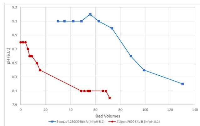
**Figure 2.** pH vs. bed volumes (data from single-pass rinsing [not recirculated]) (Source: Jacobs)
