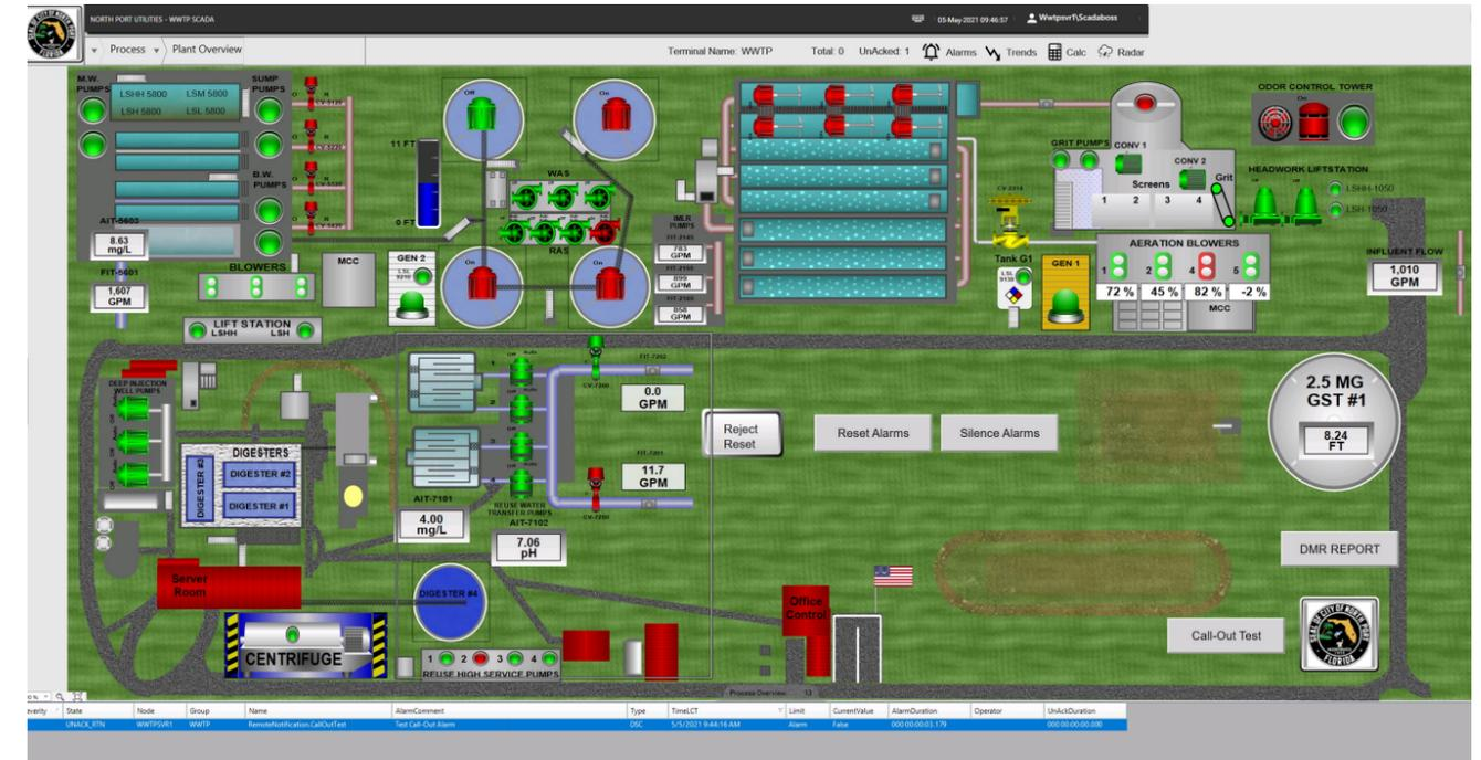
Overview of the city’s wastewater equipment connected to remote alarm notification software. When an alarm occurs on specific equipment, the City of North Port can visualize the alarms through its SCADA system.
