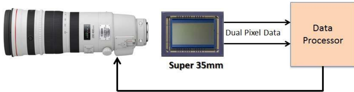
FIGURE 7: PRINCIPLE OF THE AUTO FOCUS CONTROL SYSTEM WHERE DATA FROM THE DUAL PHOTODIODES WITHIN EACH PHOTOSITE CONSTITUTES A PHASE COMPARISON WHICH IS PROCESSED TO CREATE A CONTROL SIGNAL FOR THE LENS FOCUS
