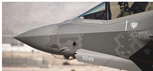
Figure 2. Electro-Optical Targeting System (EOTS) for the F-35 Joint Strike Fighter. The sensitive optical equipment is protected by a pod comprising six sheets of sapphire.
