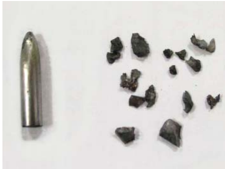
Figure 3. Before (left) and after (right): a 7.62x54R B32 API round impact versus a sapphire strike face
