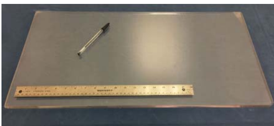
Figure 1. A sheet of EFG sapphire measuring 26 x 14 x 0.5 in 3
