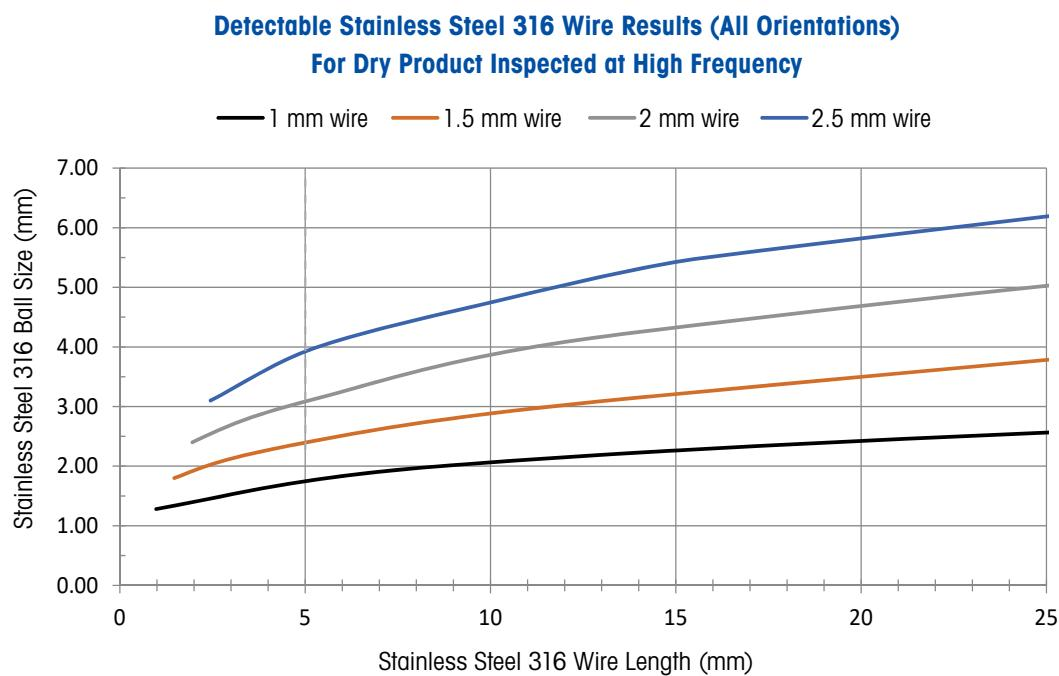
**Stainless steel is used in this example since it is typically more difficult to detect than ferrous and non-ferrous metals.**
