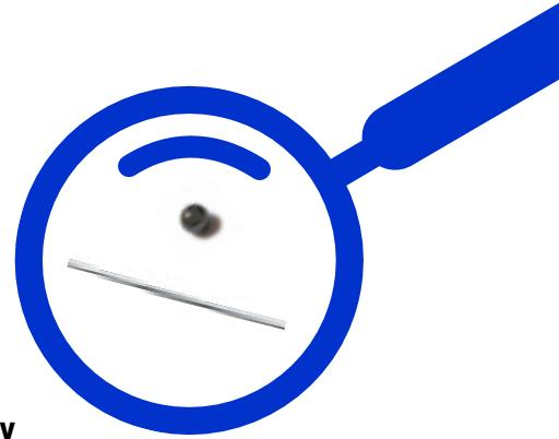
**Sensitivity is the measure of a metal detector's ability to detect a specific type and size of metal contaminant. The better the sensitivity of the metal detector, the smaller the pieces of irregular-shaped metal it can detect.**
