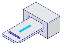
A metal detector's ability to identify a non-spherical contaminant such as wire or swarf, is partially determined by the type of metal contaminant (ferrous, non-ferrous or stainless steel), as well as the metal object's orientation. Orientation effect becomes a limiting factor when the contaminant's cross-sectional area (i.e. diameter of a wire) is less than the metal detector's spherical sensitivity.
