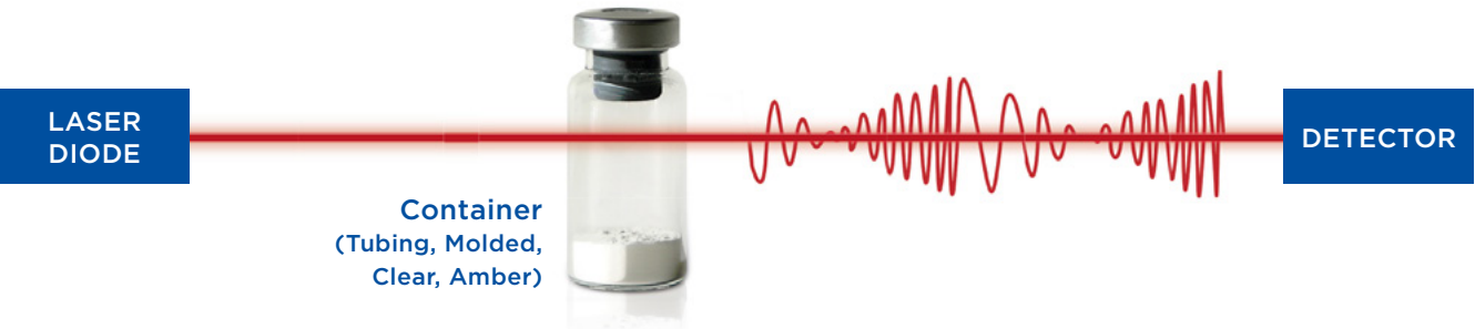
Figure 1: Non-destructive headspace analysis using a laser diode that shines through the headspace of a container.
