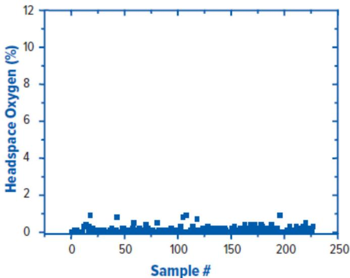
Figure 3: Headspace oxygen content of vials located in zones 4-6. Vials from this location in the freeze dryer showed no evidence of stopper pop up.
