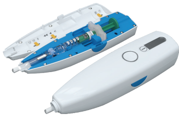
Figure 1: A therapy specific (MS) electronic injection device, to avoid severe relapses.
