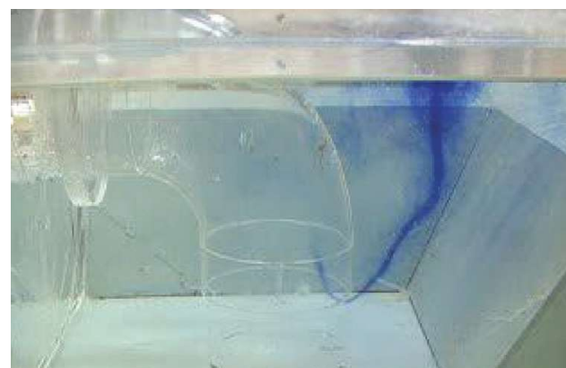
Figure 2: Surface vortex at pump 2, physical model
