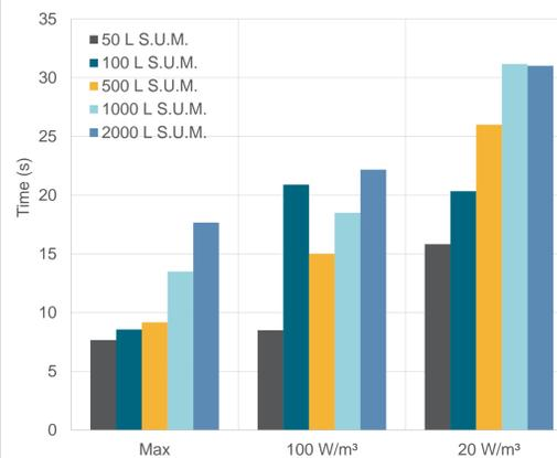
Figure 2. T95 mixing times at 2:1 volume in the HyPerforma S.U.M. at maximum PIV, 100 W/m<sup>3</sup> and 20 W/m<sup>3</sup>
