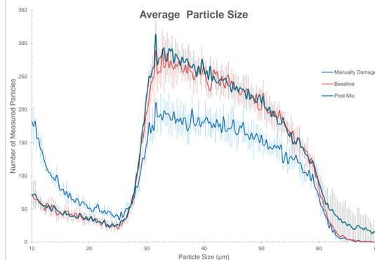
Figure 7. Particle analysis results for suspended slurry
