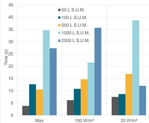
Figure 3. T95 mixing times at 5:1 volume in the HyPerforma S.U.M. at maximum PIV, 100 W/m<sup>3</sup> and 20 W/m<sup>3</sup>
