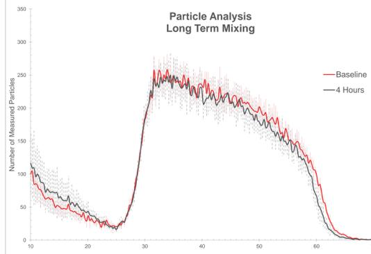
Figure 8. Particle analysis post four hours mixing
