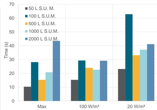
Figure 1. T95 mixing times at full volume in the HyPerforma S.U.M. at maximum PIV, 100 W/m<sup>3</sup> and 20 W/m<sup>3</sup>
