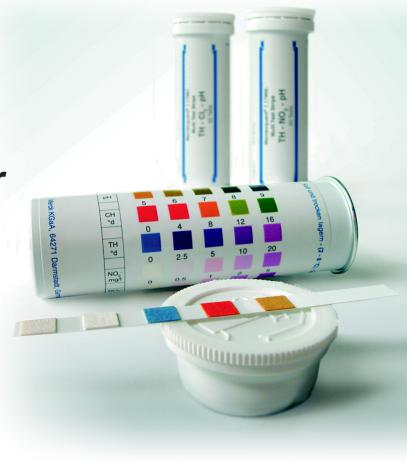
Some common uses for wastewater analysis include test strips for ammonium, nitrate, nitrite, and phosphate. Test strips for disinfection include chlorine, peroxide, and peracetic acid (PAA), a newer disinfectant for municipal effluent.
