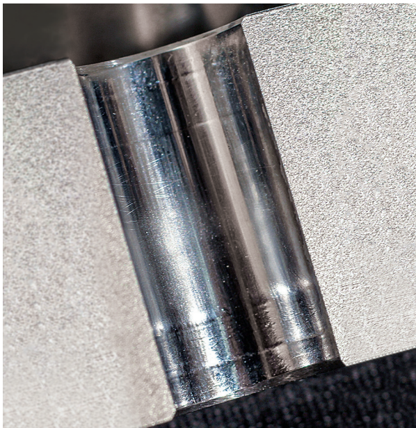
Caption: Sectioned die showing wear ring and associated punch tip wear which can result in tablet flashing.
