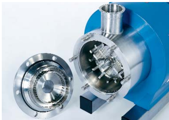
INCREASING THE NUMBER OF HOLES OR SLOTS WILL INCREASE THE ROTOR-STATOR INTERACTION AND, IN TURN, INCREASE THE NUMBER OF HIGH ENERGY REGIONS. THIS CAN BE DONE BY CHANGING THE SCREEN.
