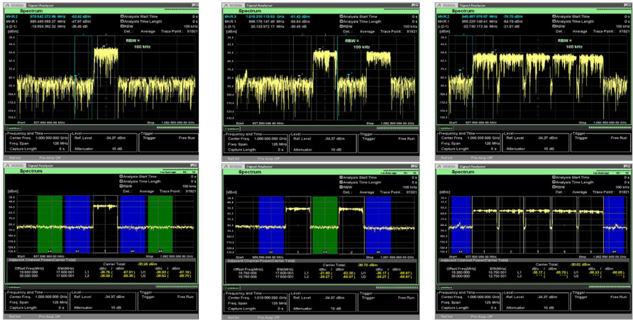
Fig 46 - ACLR Measurement on 5G waveforms
