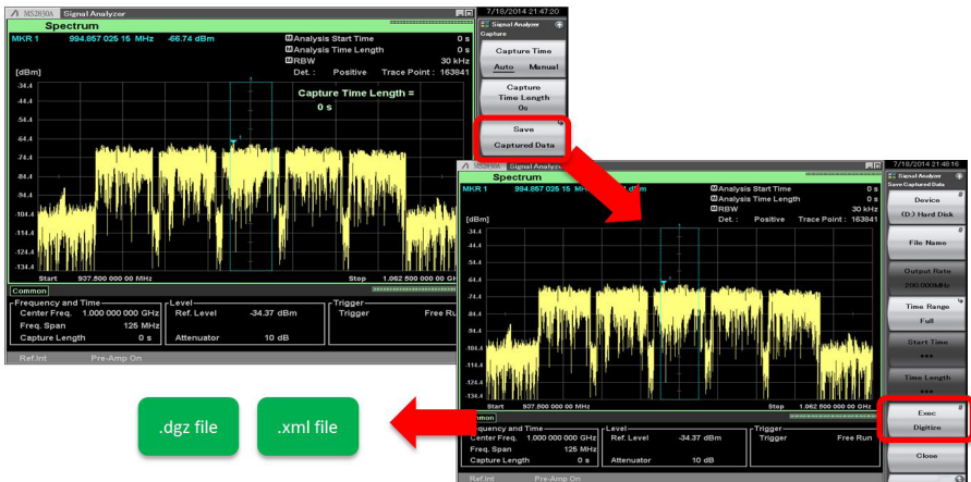
Fig 47 - Capturing real 5G waveforms with MS2830A
