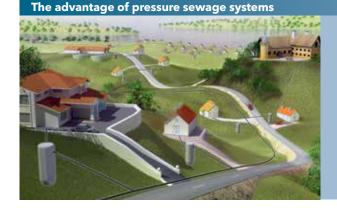
Connecting one or more pump stations to the municipal sewage network can pose distinct challenges depending on the lay of the land. Large pipes of conventional gravity systems need to be laid on a grade. Smaller pipes used for pressure sewage systems don't. This drastically cuts costs associated with excavation and construction of gravity-flow pipelines compared to pressure sewer flow pipe lines.
