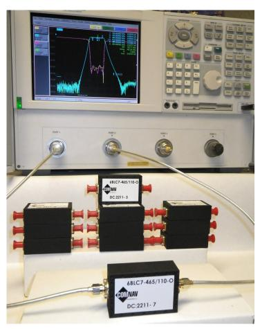
ComNav Engineering Introduces P/N 6BLC7-465/110-O. This is a high power UHF Bandpass filter with the following characteristics:
