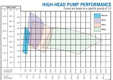
For larger flows contact the factory. Additional pump models are available up to 30" in size and up to 40,000 gpm.
