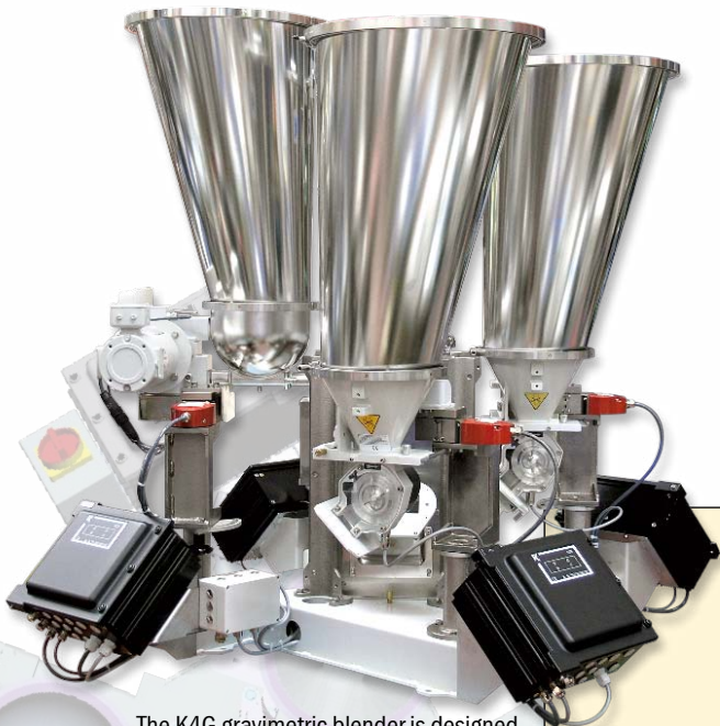
The K4G gravimetric blender is designed to group up to six feeders in a compact configuration
