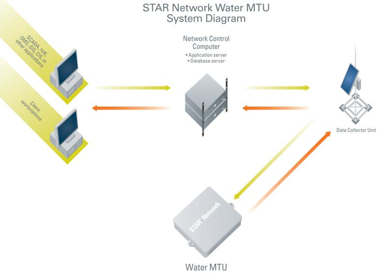
The water MTU links the meter to the STAR Network system, capturing valuable data and providing the benefits of reliable AMI.
