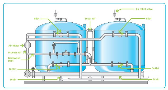
The optimal pH, and ORP (oxidation-reduction potential) are required for the correct operation of the biological process. This is achieved through the controlled injection of process air (depending on the raw water pH), which increases the ORP.
