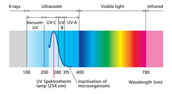
wavelength range of 254 nm, reaches the microorganisms and impacts directly on their DNA. By chan-
