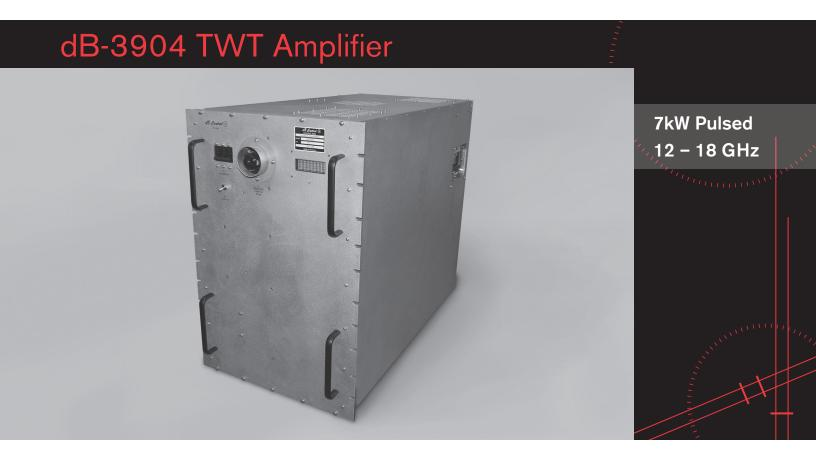
The dB-3904 power-combined traveling wave tube amplifier (TWTA) uses two wideband, periodic permanent magnet (PPM)-focused TWTs to amplify CW, AM, FM or pulse-modulated signals. Compared to a single TWT approach, the dB-3904 provides higher saturated output power and improved harmonic performance. In addition, dB Control minimizes losses from power combining by carefully matching the TWTs and other RF components for amplitude and phase over the entire frequency range.
