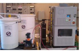
MIOX's AOP technology combines the on-site generation of aqueous chlorine and ultraviolet photoreactors to provide  $\operatorname{CL}_2/\operatorname{UV}$  AOP water treatment. During this treatment process, aqueous chlorine is first added to the water to be treated. This water is then exposed to UV light, which activates the aqueous chlorine and producing hydroxyl and other radicals. These radicals are then harnessed to destroy organic contaminants in the water.
