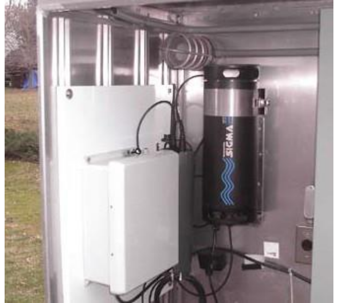
The RTUs employ switched packet protocol, which uses the Ethernet capabilities of the existing cellular infrastructure to push data in 15-minute intervals to the remote server.
