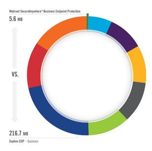
This metric compares the average amount of RAM in use by an endpoint security product during a period of system idle. This average is taken from a sample of ten memory snapshots taken at roughly 60 seconds apart after reboot. Products with lower idle RAM usage are considered better performing products in this category.
