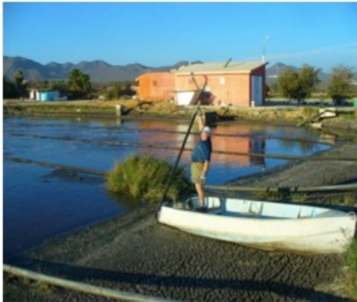
Figure 2 – A sludge measurement approximately five feet from the shore of the lagoon measured over 7 feet of sludge depth. This depth was very consistent around the edges of most of the lagoon.
