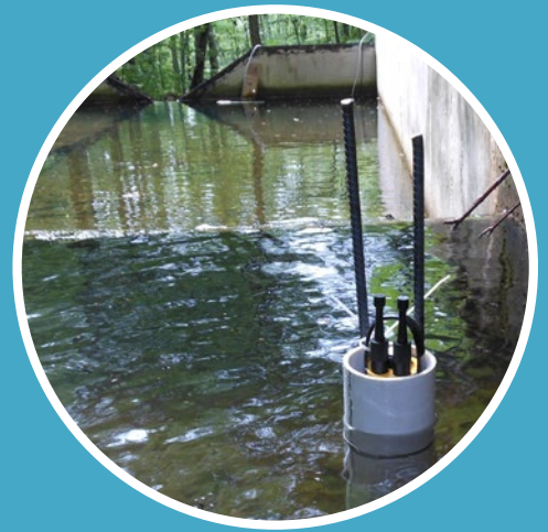
Sondes can be left out long-term to monitor key water quality interactions.
