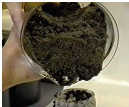
Fig. #6 - Polymer Thickened Sludge (~5% TSS)
