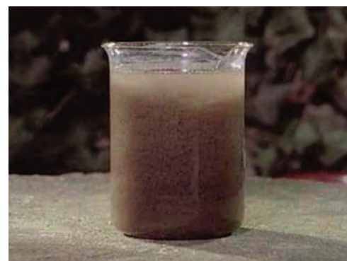
Fig. #2 - Suspension of Activated Sludge
