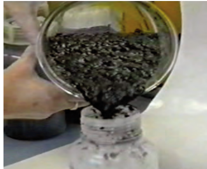
Fig. #5 - Statically Thickened Sludge (~5% TSS)
