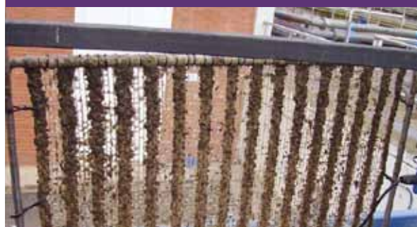
Cleartec ® media showing fixed biomass when pulled out the water
