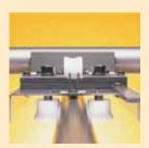
The suction header is locked onto the guide rail with rollers to prevent disruptive derailments
