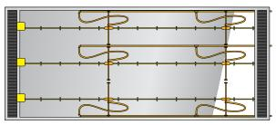
The Leopold CT2 sludge collection system can be designed to accommodate extra-wide sedimentation tanks. And each track can be separately controlled to vary the number of passes and the speed of each pass.
