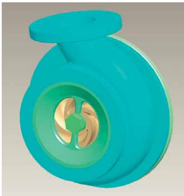
Geometry of a typical casing, impeller, and cutter bar assembly for a centrifugal pump with a chopping action between the impeller and the suction plate.
