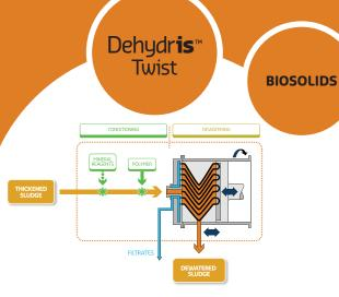
Based on proven Bucher Unipektin piston press technology (with more than 2,000 food industry references), Dehydris™ Twist represents one of the most innovative and efficient systems in the dewatering market.
