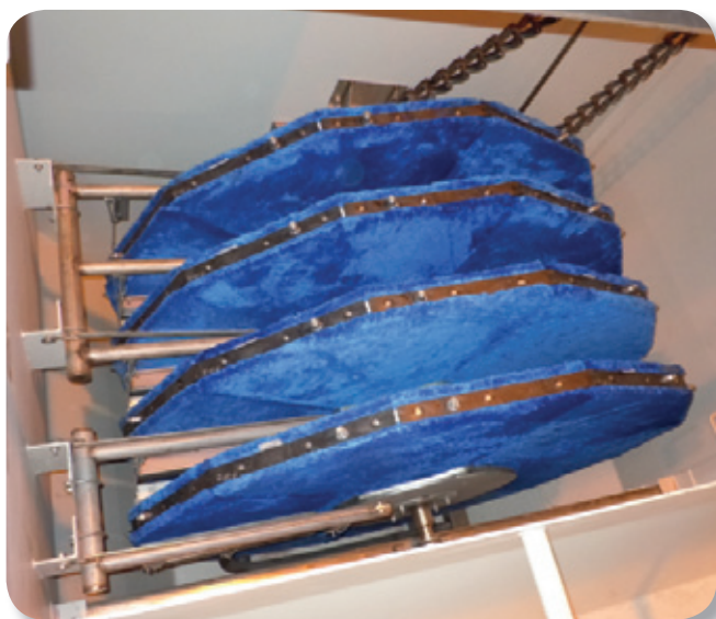
An AquaDisk® filter with Microfiber cloth treats cooling tower blow-down.
