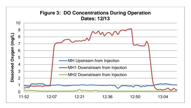
In addition to the above, the analytical data also shows an average BOD reduction of ~20% with a corresponding ~8% decrease in COD. Therefore, unlike competing technologies which address odor problems with chemical solutions that typically increase solids loading at wastewater treatment facilities, oxygen injection has the potential to reduce loadings at treatment facilities, effectively offsetting some operational costs while simultaneously increasing the expected lifespan of those facilities.
