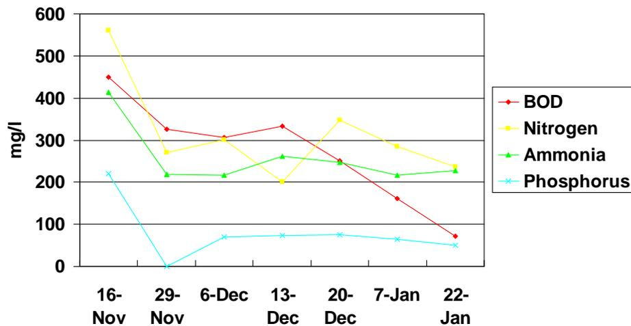
**Figure 4:** Water quality data of the surface water of the hog lagoon during the 60 day trial. In every case, the reduction was at least 50%, with nitrogen and phosphorus exhibiting close to an 80% reduction
