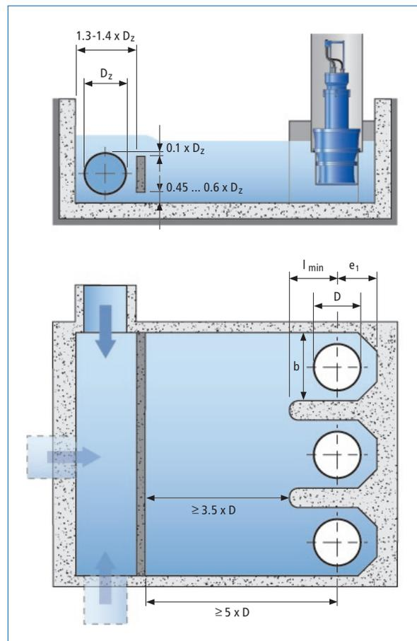
Fig. 2.3-c: Example of a pump station with cross flow and curtain wall
