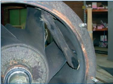
Fig. 2.7-d: Wood inside the diffuser casing of an Amacan pump
