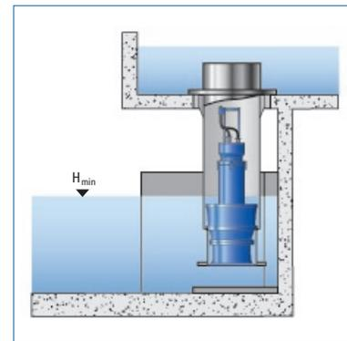
Fig. 3.1-c: Installation type BU
