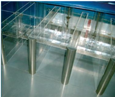
Fig. 2.5-a: Acrylic model of an Amacan P pump station
