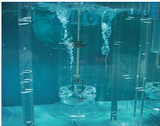
*Fig. 2.1-a: Vortices developing as a result of unacceptable approach flows into the chamber – jet directly impinging on discharge tube*
