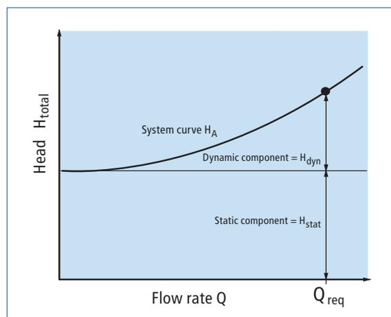
Fig. 1.2-a: Example of a system curve [ $H = f(Q)$ ]
