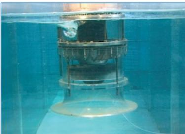
Fig. 2.5-f: Laboratory photo of a surface vortex type 3
