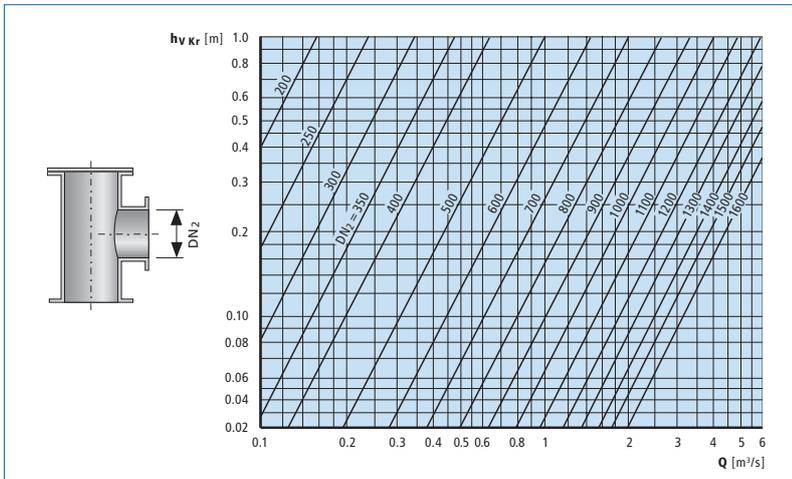
Fig. 1.2-d: Determining the pressure loss in a discharge elbow outlet
