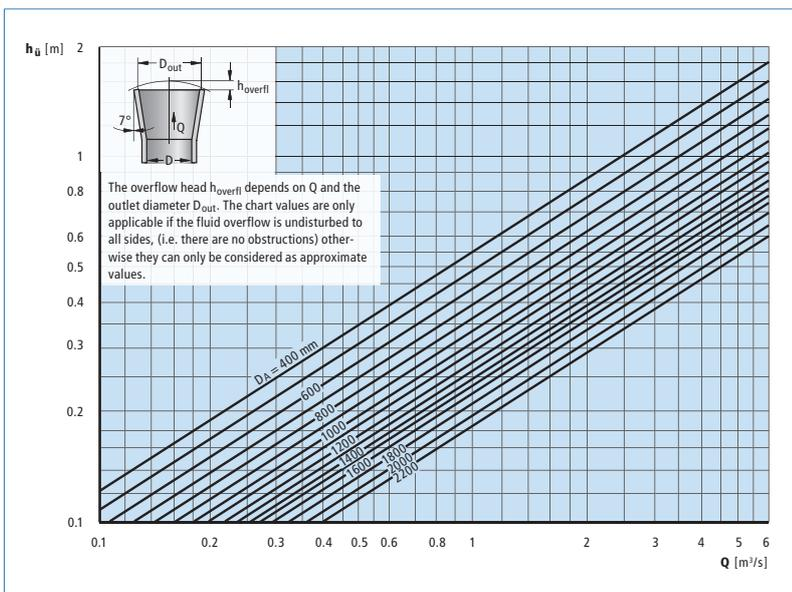
Fig. 1.2-e: Establishing the overflow head  $h_{overfl}$
