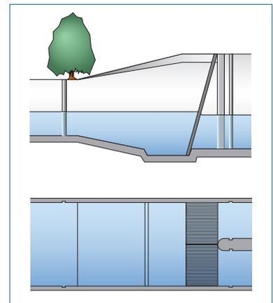
Fig. 2.7-c: Shingle trap upstream of pump station
