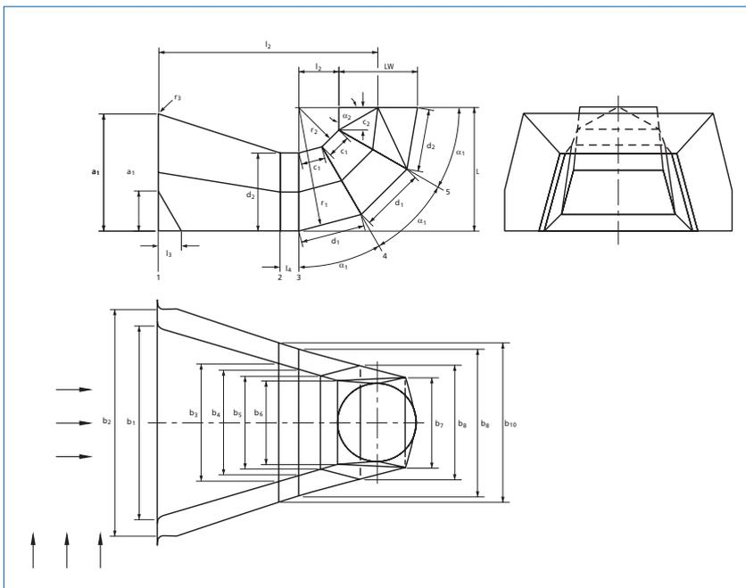
Fig. 2.2.4-h: Variant of a segmental bend
