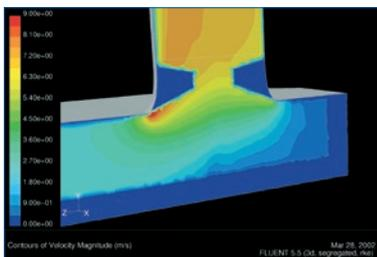
Fig. 2.6-b: Simulation of approach flow to discharge tube
