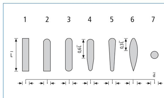
Fig. 2.7-g: Different shapes of screen bars
