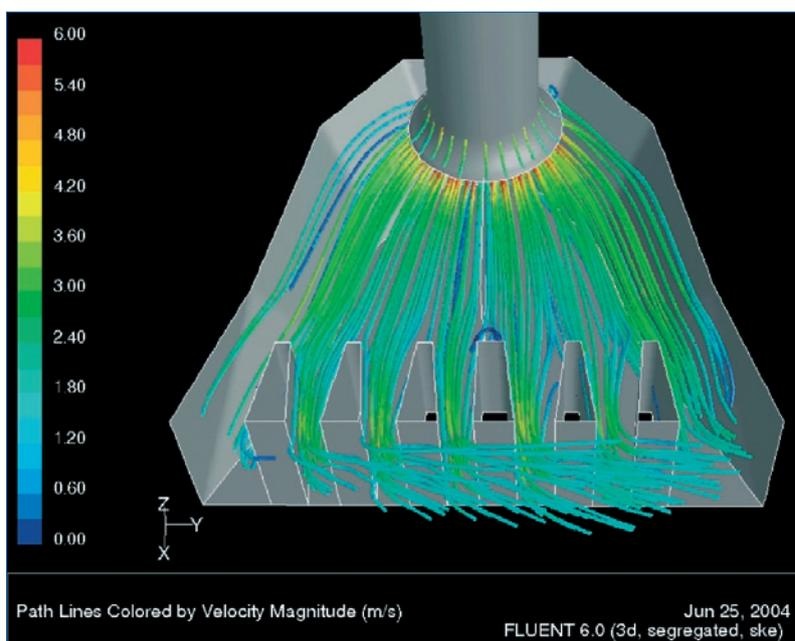
Fig. 2.4-a: Specially dimensioned intake chamber for cross flows of  $v = 1,8\text{ m/s}$
