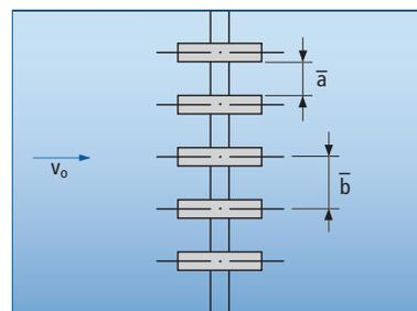
Fig. 2.7-f: Screen layout drawing
