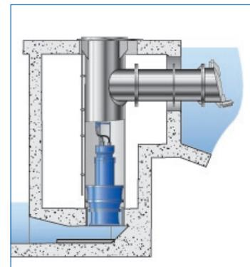
*Fig. 2.2-c: Variants of discharge tube design with underfloor discharge nozzle*
