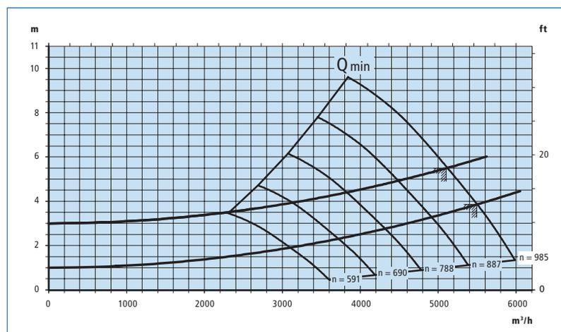
Fig 1.3-a: Amacan P 800 - 540 A 4 with speed curves
