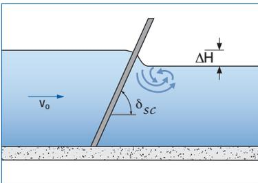
Fig. 2.7-e: Flow through screen, without lowered floor
