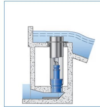
*Fig. 2.2-a: Variants of discharge tube design with free discharge*
