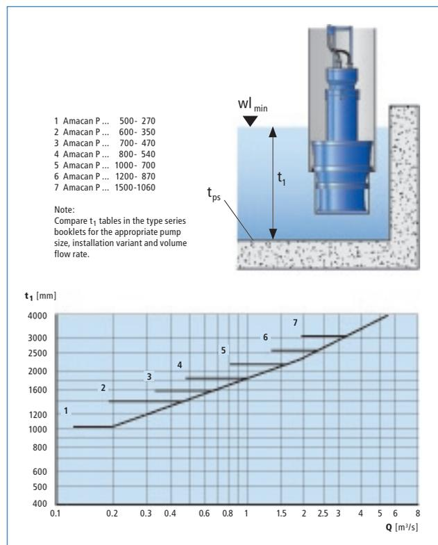
Fig. 1.2-c: Calculation of the minimum water level  $t_1$  for Amacan P (for Amacan K and Amacan S refer to the appropriate type series booklet)
