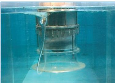
Fig. 2.5-e: Laboratory photo of a surface vortex type 6
