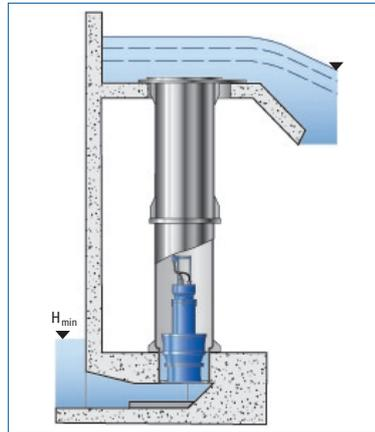
Fig. 3.1-a: Installation type A
