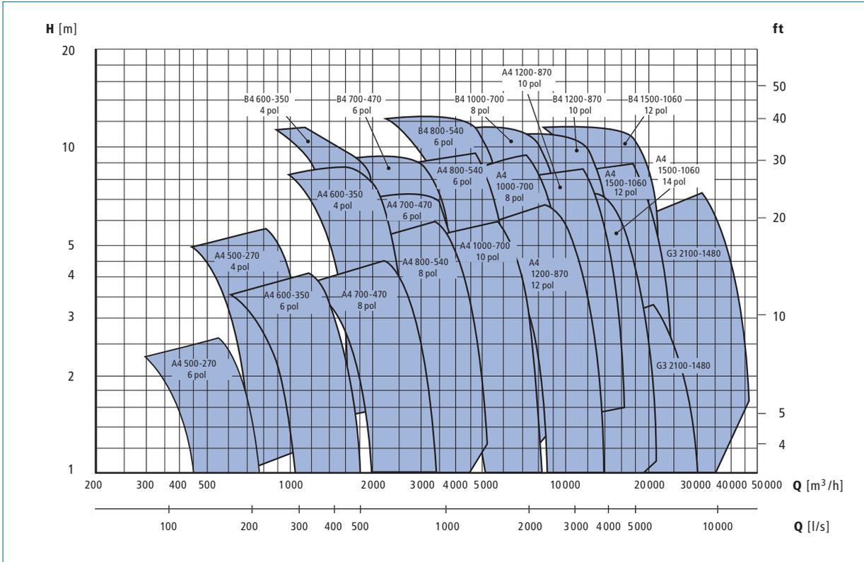
Fig. 1.1-b: Selection chart Amacan P pumps (50 Hz)
