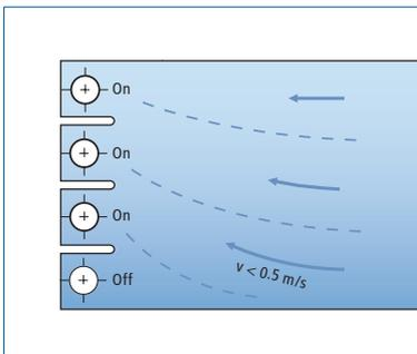
Fig. 2.3-d: Flow pattern developing with variable pump operation
