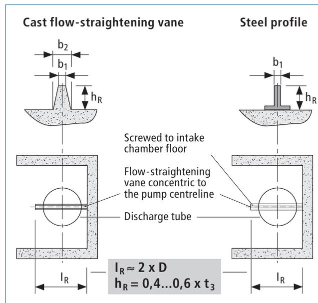
Fig. 2.2.4-c: Sizing the flow-straightening vane
