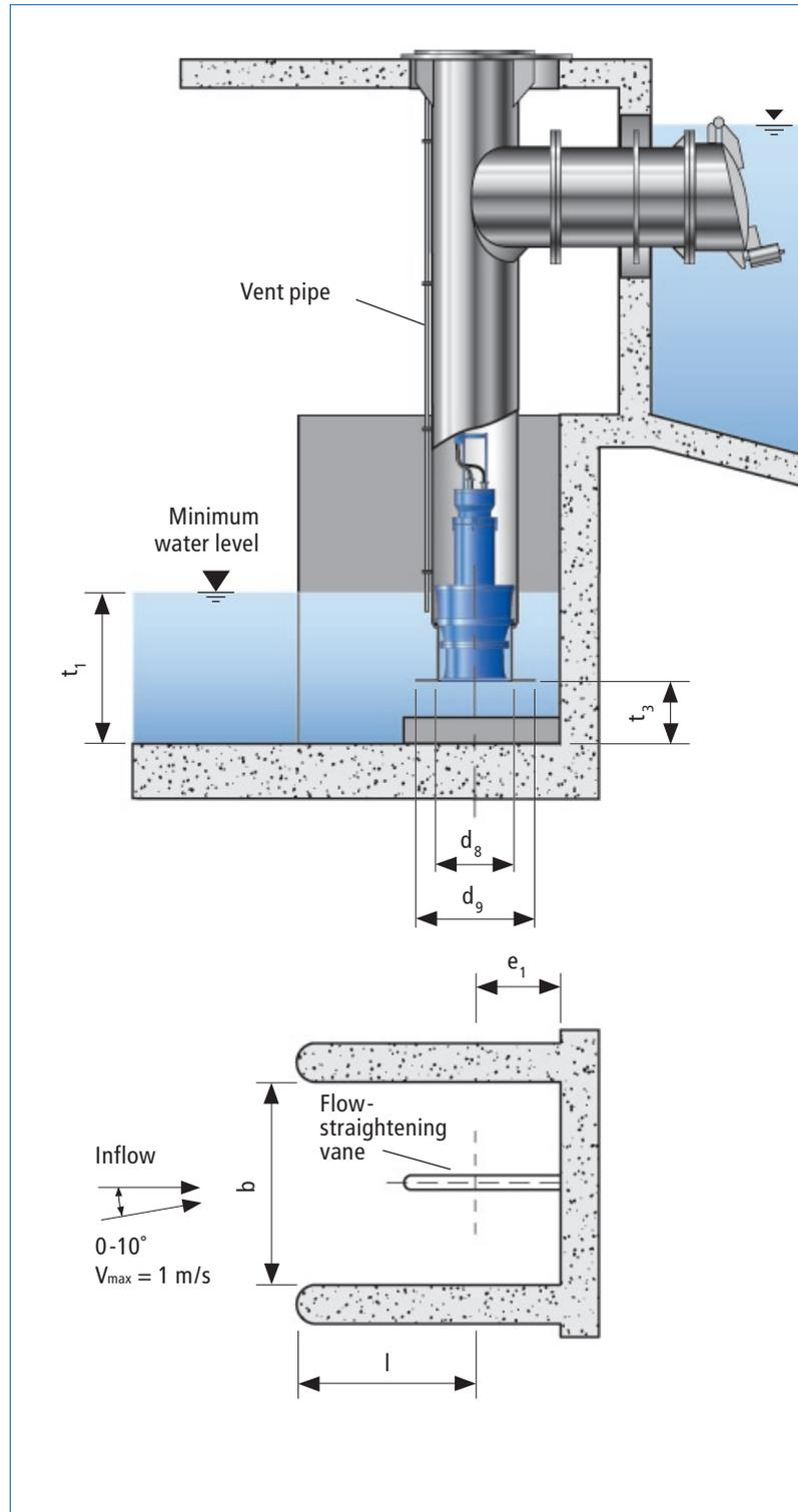
Bild 2.2.2-a: Open intake chamber with suction umbrella
