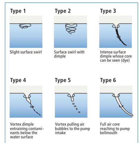
Fig. 2.5-c: Classification of surface vortices according to Hecker (Types 1 to 6)
