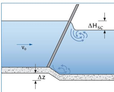
Fig. 2.7-b: Flow through screen with lowered floor
