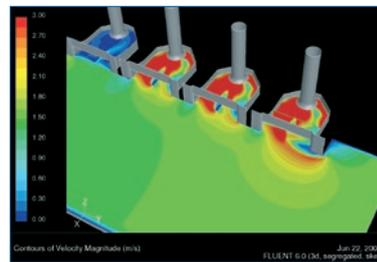
Fig. 2.6-c: Simulation of pump station with several pumps
