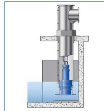
*Fig. 2.2-b: Variants of discharge tube design with above-floor discharge nozzle*
