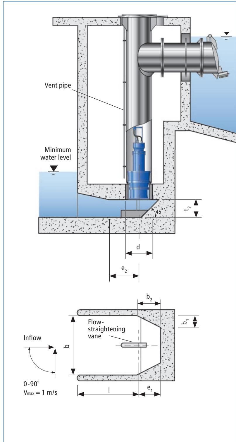
Fig. 2.2.3-a: Covered intake chamber
