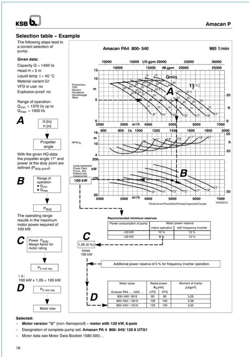
After the system curve has been determined, this should always be plotted together with the pump characteristic curve in order to check the operating points (curve intersections). In this way, the designer can ensure that no operating conditions outside the permissible section of the characteristic curve arise.
