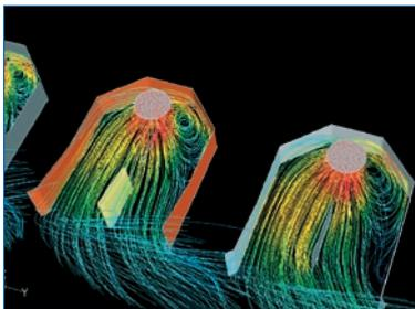
Fig. 2.6-a: Flow patterns in Amacan intake chambers
