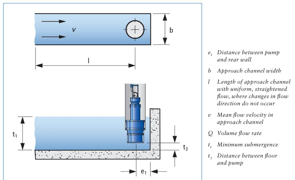
Fig. 2.2-e: Important intake chamber data (for actual dimensions refer to the type series booklet or selection software)
