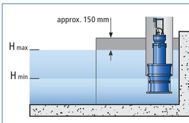
Fig. 2.2.4-a: Chamber wall height
