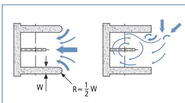
Fig. 2.2.4-b: Chamber intake design
