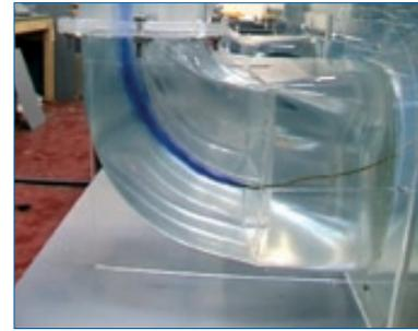
Fig. 2.2.4-i: Variant of a double elbow in a model test
