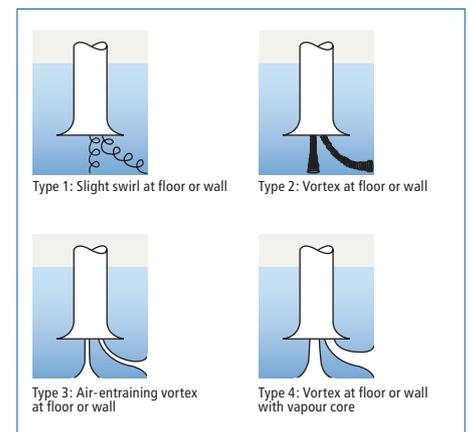
Fig. 2.5-d: Classification of submerged vortices according to Tillack (Types 1 to 4)
