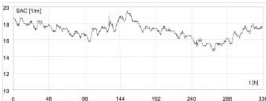
Fig 8: Progress graph of SAC over time at the outlet of a wastewater plant
