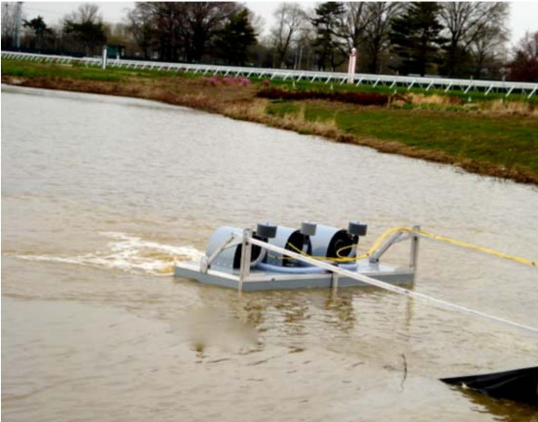
Figure 2 – Reliant Water Model WQA Water Moving aerator in racetrack lagoon.
