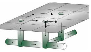
1D elements may be integrated into a 2D flow area to accurately model 1D flow. Cells underlying natural channels that are modeled in 1D are made inactive to avoid double calculation of conveyance and volume.
