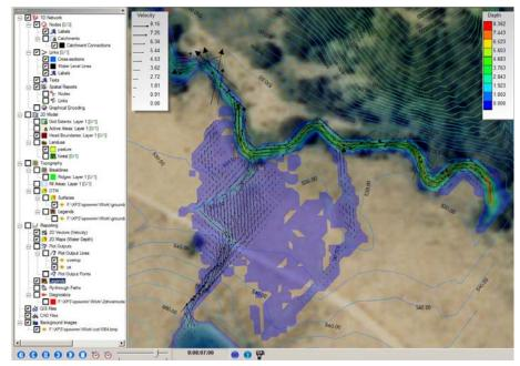
Time series outputs of water depth and velocity at user defined points or flows across user defined polylines are easily generated. These plots may be displayed, printed or exported as graphic files.
