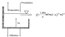
The unit hydrograph methods such as SCS, SBUH, LA County Modified Rational, etc. are primarily used for single event simulations. The SWMM runoff method is a deterministic hydrologic method suitable for comprehensive analysis and design including the simulation of LID (WSUD) using catchment surface redirection capabilities.
