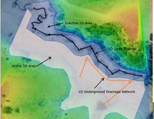
The flood plain is represented as an Active 2D Area polygon. It borders the 1D open channel which is represented as a 2D Inactive Area. The 1D underground drainage network is added to the model.
