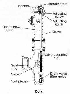
Another type of dry barrel hydrant, the "Cory type" has a main valve that closes against the water pressure. In this hydrant the threaded portion of the operating stem is located down inside the waterway. A toggle mechanism acted upon by opposing threads moves the main valve into and out of the valve's seat area. This type is distinctive by having the operating nut located off-center on the bonnet.
