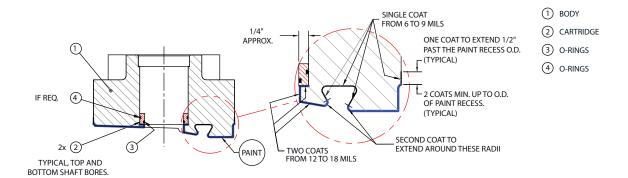
PrattGuard 200 is a cross-linked epoxy-phenolic cured with a polyamine curing agent. 75% solids content, by volume. It's excellent overall chemical resistance to a broad range of damaging acids, alkalies and solvents make it the perfect choice for use in extreme-condition applications.
