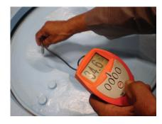
The joints between the disc rolled edge, the disc edge, and the seat groove were considered critical in this test. None sustained any damage, as the PrattGuard 200 coating had not allowed salt
