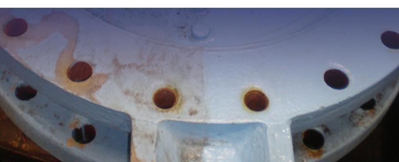
A report on a test, its results, and conclusions following the saline spray exposure of a Pratt 24-inch Butterfly Valve coated with PrattGuard 200 on critical surfaces. The valve body and disc, which are of ductile iron construction (ASTM A-536 (65-45-12) had seals added to the valve body and disc shaft bores via additional machining, to prevent intrusion of the flow media into these areas.
