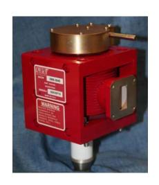
The VMX3045 is a high power, coaxial pulsed magnetron that provides up to 400kW of peak output power and 400 W of average output power at .001 duty cycle and 3.5 uS pulse width. The VMX3045's combination of high power and small size, make it ideally suited for mobile linear accelerators.
