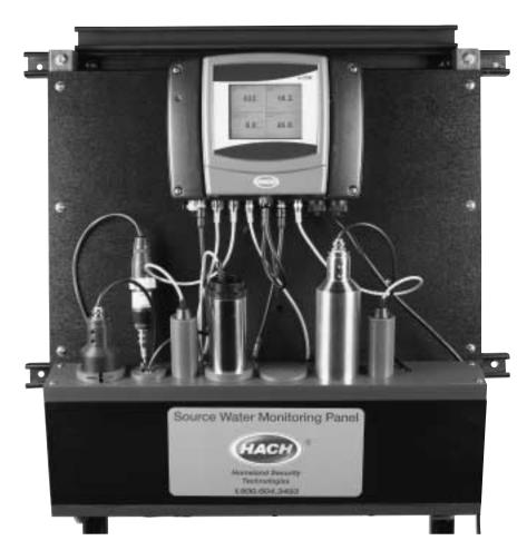
Source waters can be vulnerable to an accidental or intentional contaminant events. Monitoring an input water source can provide useful information to the Drinking Water Plants that process incoming water. Plants can shut their intake down should their Source Water Panel parameters change significantly.
