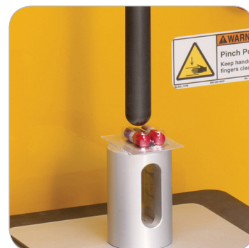
Figure 2: Blister Pack Support Fixture Used for Tablet/Capsule Extraction Test
