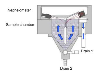
The sample enters at the sample inlet. A constant head guarantees a constant sample flow into the sample chamber. Excess sample overflows directly into drain 1. The sample flows into the sample chamber, fills it, and overflows into drain 1. The LED beam impinges continuously on the sample surface.
