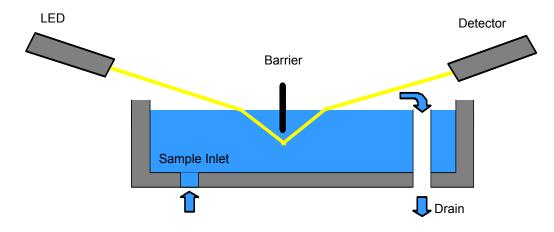
The LED white light source transmits light through the water sample to a photo-electric detector. The source and the detector are at a 90 degree angle, with a barrier in place to prevent any surface light refractory. The detector measures the incoming scattered light. A second detector is located at the LED source to measure intensity. An algorithim is used to calculate turbidity based on the intensity of both signals.
